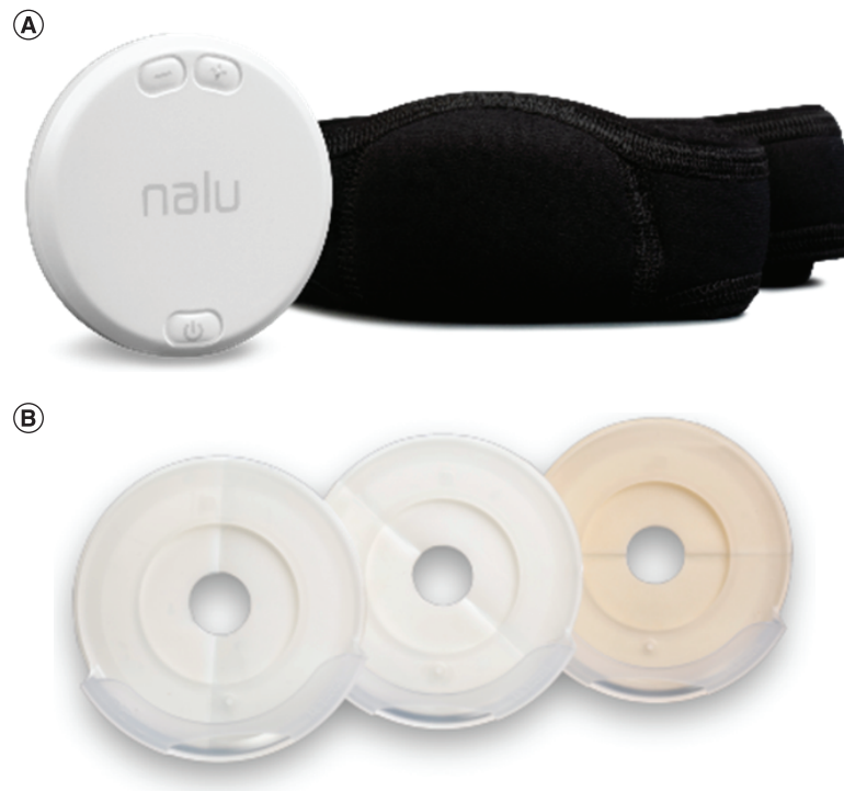
Figure 1. Nalu™ Neurostimulation System therapy disc, adhesive clips and optional belt. (A) The therapy disc powers and controls the implantable pulse generator wirelessly using inductively coupled radiofrequency energy. (B) The therapy disc is held in place by an adhesive clip applied to the skin. Alternatively, it can be held in place by a belt/cuff worn over clothing; this is shown adjacent to the therapy disc in (A).
