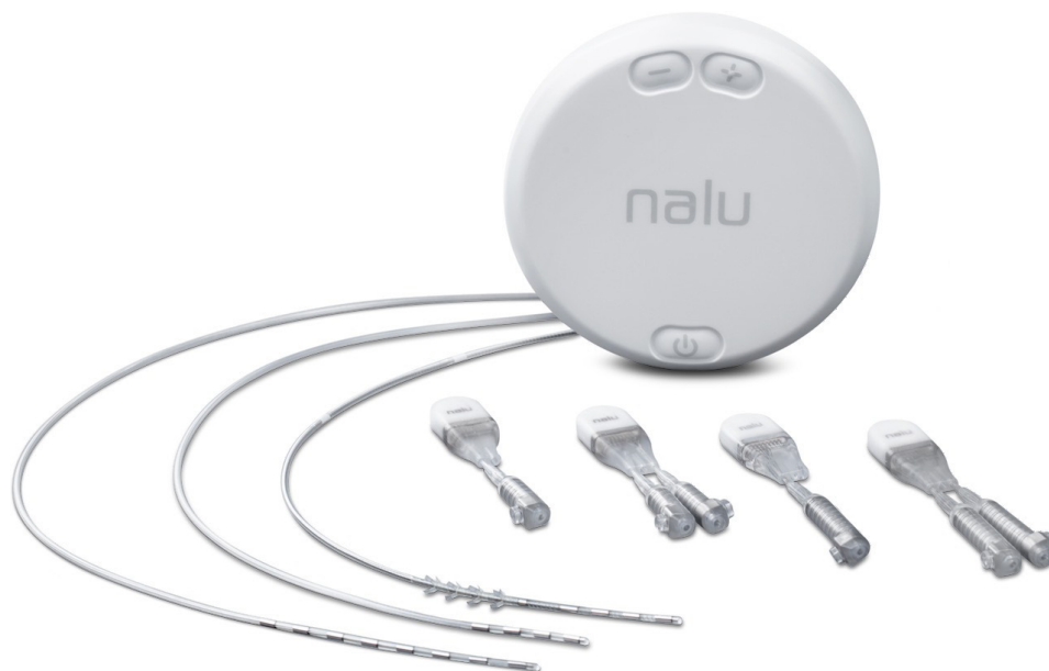
Figure 4 Peripheral nerve stimulation system used during the course of this study. The Nalu system consists of a micro-implantable pulse generator (<1.5 cc) that is powered by a therapy disc worn over the implant with an adhesive clip or a limb cuff. Bidirectional telemetry allows for optimal therapy delivery. There were three lead configurations employed during this study: four-contact leads with tines, four-contact leads without tines and eight-contact leads without tines. In addition, there were four micro-IPG configurations: Single port for four-contact leads, dual port for four-contact leads, single port for eight-contact leads and dual port for eight-contact leads.
